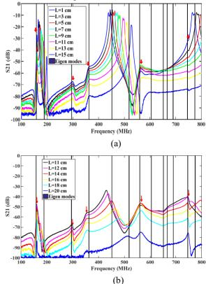
Figure 3: Measured  $S_{21}$  for different values of L (L is shown in Fig. 2) without (a) and with (b) absorbing material in the beam pipes of the BGI monitor.
