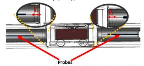
Figure 2: Cut-away view of the BGI monitor with long electric probes inside the beam pipes. The distance between the entry of the BGI tank and the probe is L (see the figure inset).
