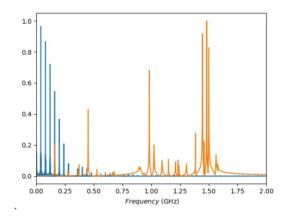
Figure 6: Normalized power density spectrum of the PS beam in blue, and normalized  $Re [Z_{||}]$  in orange.
