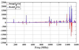
Figure 5: Real and imaginary part of  $Z_{\parallel}$  (simulated using CST [3]).
