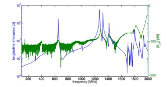
Figure 4: Comparison of S-parameter transmission measurement with calculated impedance spectrum of the VVSA.
