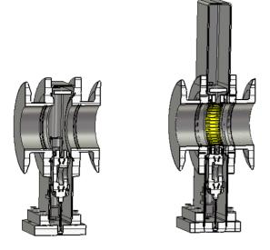
Figure 2: CAD model of a VVSA sector valve (left) and the impedance shielded version (right). The body of the shielded valve version is significantly larger than the unshielded one. The extended size is required for housing the impedance shield if the valve closes.
