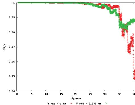
Figure 6: Polarization in the RCS on the ramp for different values of the RMS orbit error. Only the latter part of the ramp is shown here for better visibility. No depolarization occurs in the earlier part.
