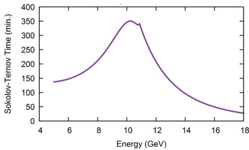
Figure 4: Sokolov-Ternov self-polarization time in the eRHIC electron storage ring as function of beam energy.
