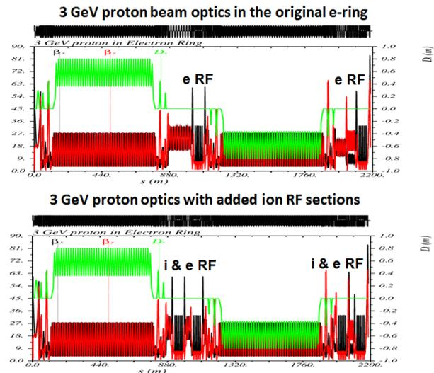
Figure 3: 3 GeV proton beam optics in the e-ring before and after adding the ion rf sections.
