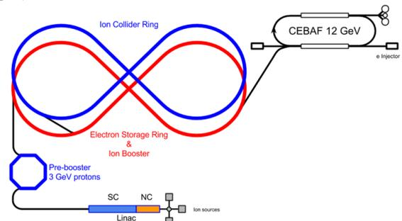
Figure 1: Layout of the alternative JLEIC design.
