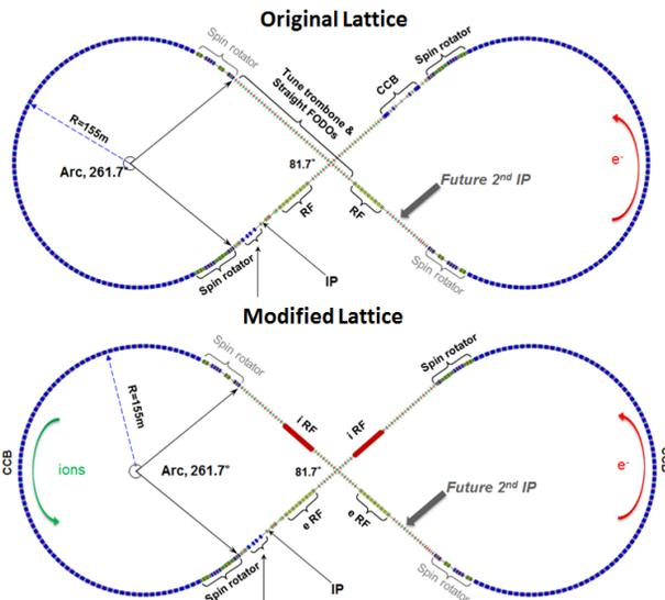
Figure 2: e-ring lattice before and after adding ion rf sections.
