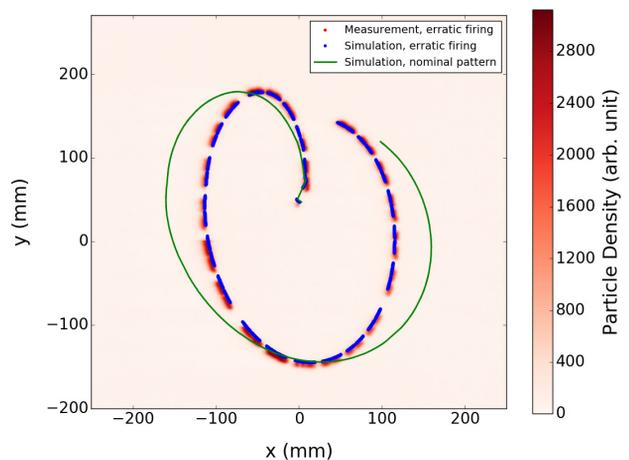
Figure 1: Simulated bunch pattern (blue) and measured distribution at the BTVDD screen (red) for an abnormal dump event on October 1, 2016 due to the spontaneous firing of one horizontal dilution kicker of Beam 1. For comparison, the simulated bunch pattern for a nominal dump is depicted in green. Note that the simulated data was scaled by a factor 1.04 in the vertical plane.
