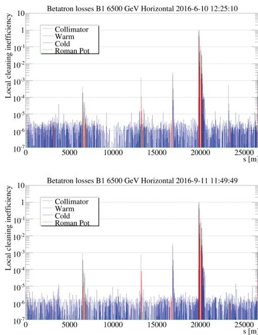
Figure 2: Loss maps measured for B1H at  $\beta^* = 40$  cm: nominal (top) and ATS pre-squeezed (bottom) optics.
