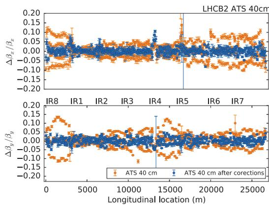
Figure 1: Hor. (H) and vert. (V)  $\beta$ -beating measured at  $\beta^* = 40$  cm (example for beam2) before and after (global) correction. A local correction knob (triplet quadrupole trims) was preset based on the 40 cm nominal optics.
