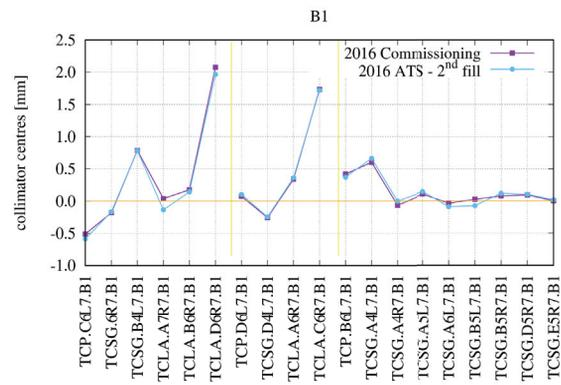
Figure 3: IR7 collimator centers measured for beam1: nominal vs. ATS optics at  $\beta^* = 40$  cm.
