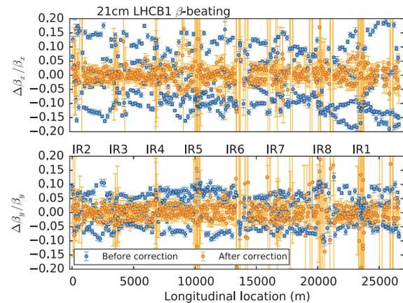
Figure 4: H and V  $\beta$ -beating measured at  $\beta^* = 21$  cm (example of beam1) before and after (global) correction.
