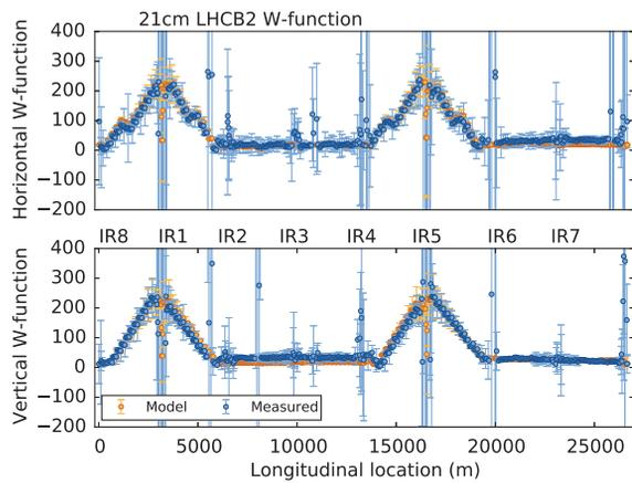
Figure 5: H and V Montague functions measured at  $\beta^* = 21$  cm (example of beam2).  $W \equiv 100$  units corresponds to an off-momentum peak  $\beta$ -beating of 20% at  $\delta_p = 10^{-3}$ .
