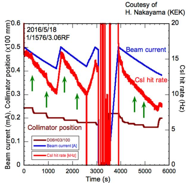
Figure 6: Background suppression using a collimator named D06H3 in LER. Collimator position refers to the aperture of the collimator in an outside axis of the ring.
