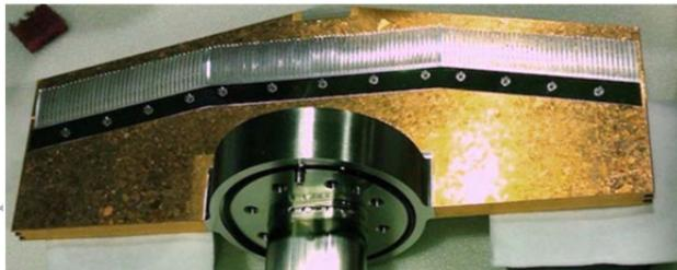
Figure 3: Moveable jaw with RF fingers.
