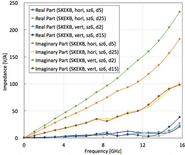
Figure 5: Real and imaginary parts of the impedances of collimators for a bunch length of 6 mm. *d* refers to an aperture.
