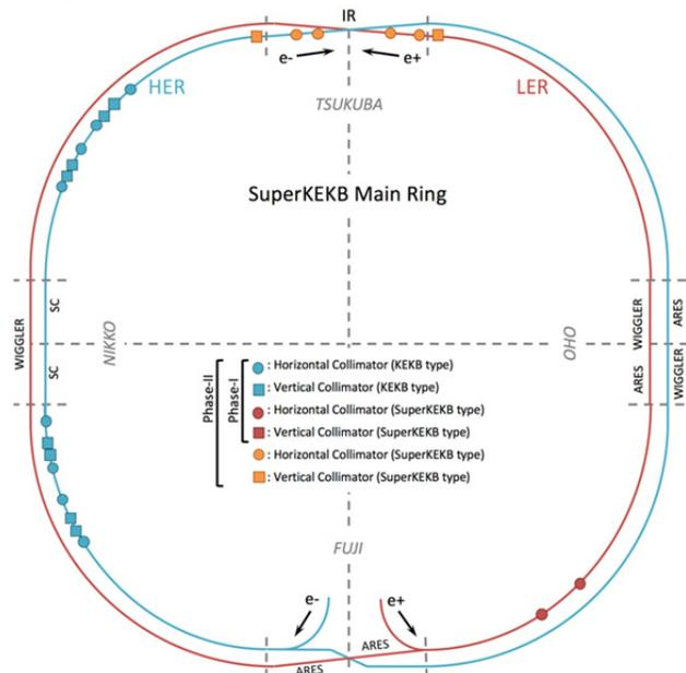
Figure 1: Collimators location in the phase-1 and -2 commissioning.
