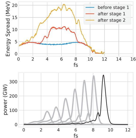
Figure 4: The energy spread (top) of an electron beam before the first stage, before the second stage, and after the second stage in the non-fresh slice scheme. With an optimal delay, the peak power increases from 90 GW to 350 GW (bottom) after a six undulator second stage. The power before the first undulator and after each of the six undulators is shown, with the black trace indicating the power after the last undulator.
