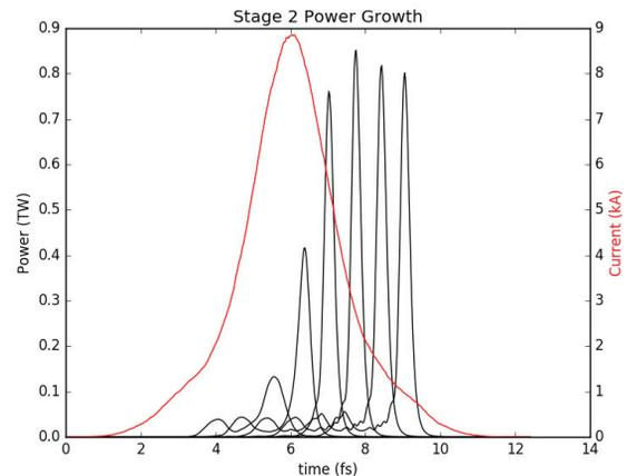
Figure 5: The power growth (black) and current (red) in the second stage of a fresh slice, two stage simulation. The power after each of the six undulators is shown. With fresh electrons to lase with, the x-ray power approaches 1 TW after the second stage. This simulation was conducted at 800 eV.
