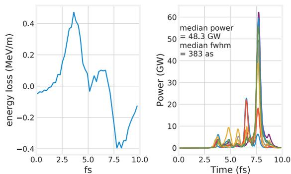
Figure 3: The longitudinal energy loss due to space charge in an overcompressed beam (left), and the resultant x-ray pulses (right) from eight simulations. This space charge force chirps the beam. A reverse taper is applied to the undulator in order to match the positively chirped parts of the electron beam.
