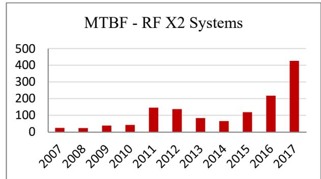
Figure 4: MTBF(hrs) by year for both installed Rf systems cavity and RF amplifiers combined.
