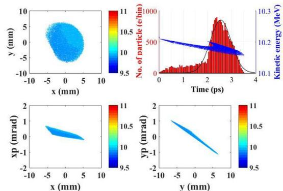
Figure 3: Simulated transverse and longitudinal particle distributions at the TR experimental station.
