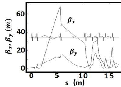
Figure 5: Simulated transverse betatron functions from the RF-gun exit to the undulator entrance.
