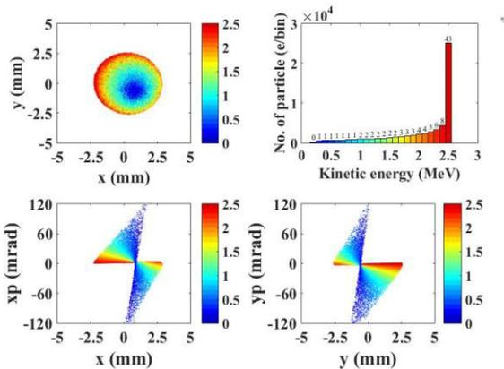
Figure 2: Simulated transverse phase space distributions and energy spectrum at the RF-gun exit. Different colors in the plots represent the particles with different energies in MeV unit.
