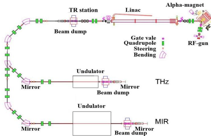
Figure 1: The planned layout of the electron beam injector system and the linac-based MIR/THz FEL Beamlines at the Plasma and Beam Physics (PBP) Research Facility, Chiang Mai University, Thailand.
