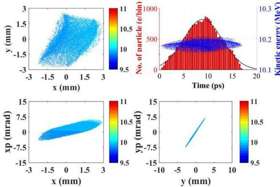
Figure 4: Simulated longitudinal and transverse phase space distributions at the undulator entrance.
