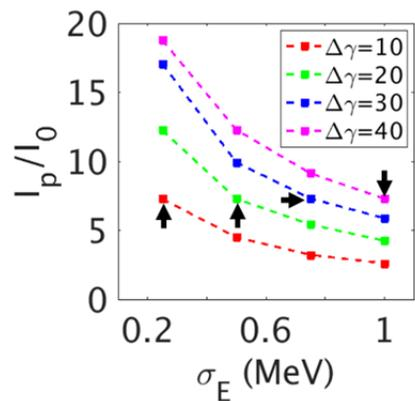
Figure 7: The normalized peak current of the current spike, which has the minimum width (Fig. 6) with respect to the slice energy spread.
