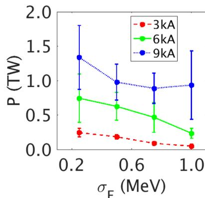
Figure 8: Maximum radiation peak power at the end of undulator line for different base current with respect to the slice energy spread of the electron beam.
