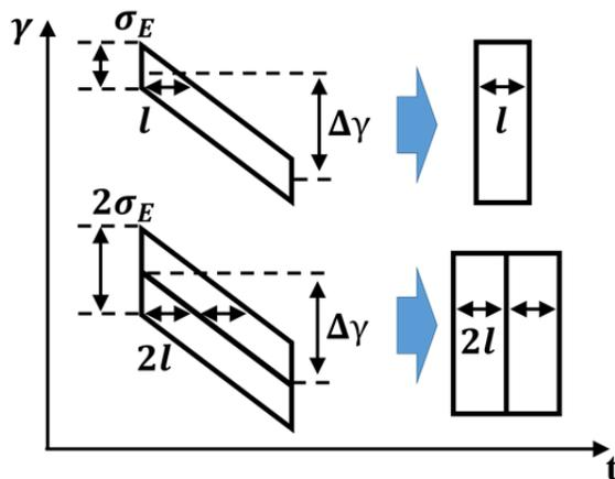
Figure 3: Schematic representation of the bunch compression in ESASE scheme for two cases which have the same energy difference ( $\Delta\gamma$ ) and different slice energy spread (up:  $\sigma_E$ , down:  $2\sigma_E$ ).
