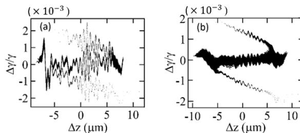
Figure 2: Bunch length – energy phase space at the PAL-XFEL linac end (a) without laser heater and (b) with laser heater.
