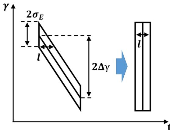
Figure 4: Schematic representation of the bunch compression in ESASE scheme for the case, which has  $2\Delta\gamma$  energy difference and  $2\sigma_E$  slice energy spread.
