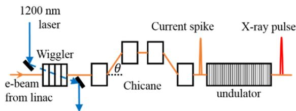
Figure 1: Layout of the ESASE scheme.
