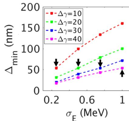
Figure 6: The minimum width of the current spike with respect to the slice energy spread.
