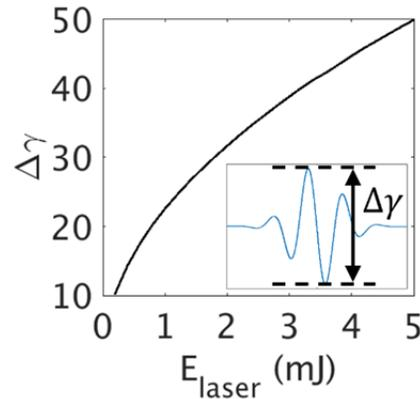
Figure 5:  $\Delta\gamma$  (see inset) after the wiggler with respect to the laser energy when the laser wavelength is 1200 nm. Inset: modulated electron beam energy along the bunch length after the wiggler.
