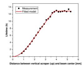
Figure 1: Lifetime vs. distance between the vertical scraper and the beam centre for tuned Landau cavities.
