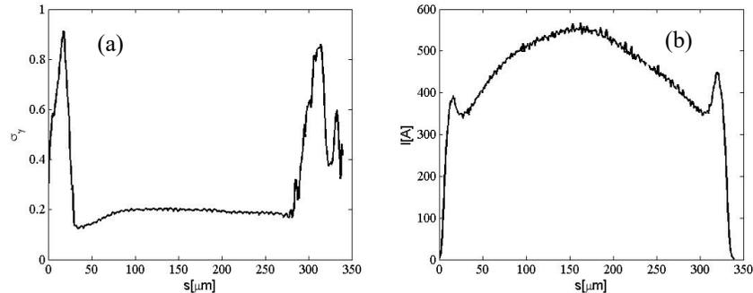
Figure 2: The output electron beam from elegant (a) energy spread, and (b) current profile.
