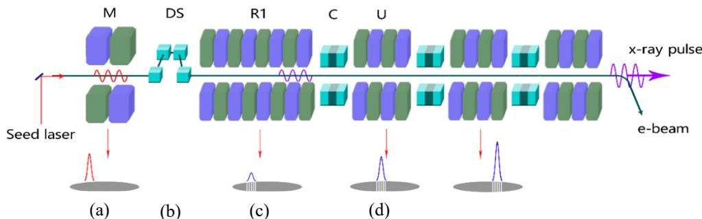
Figure 1: Schematic view of HB-HGHG scheme (a) Modulator (M), (b) Chicane (DS), (c) Short radiator (R1), (d) Chicane-Undulator (C-U) modules.
