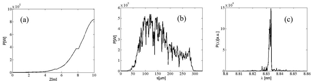
Figure 6: (a) the FEL gain curve, (b) the radiation peak power and (c) the output spectrum at the final Radiator of the conventional EEHG scheme.
