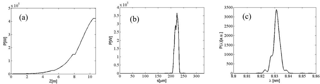
Figure 5: (a) the FEL gain curve, (b) the radiation peak power and (c) the output spectrum at the exit of the two-stage cascaded HGHG scheme.
