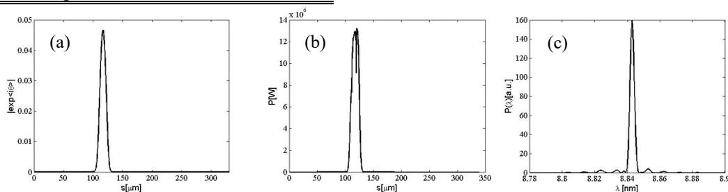
Figure 3: (a) Bunching factor at the entrance of short Radiator, (b) the output radiation peak power and (c) the output pulse spectrum from the short radiator.
