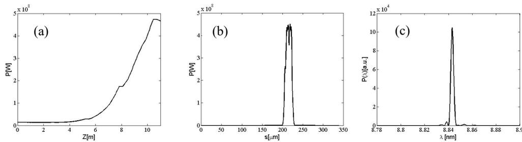
Figure 4: (a) the FEL gain curve, (b) the radiation peak power and (c) the output spectrum of the HB-HGHG scheme in one C-U module.
