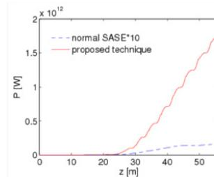
Figure 4: FEL peak power gain curves for normal SASE (blue dashed line) and the proposed scheme (red solid line).
