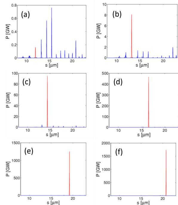
Figure 3: XFEL radiation structure evolutions along the undulator beamline at the end of (a) the 1<sup>st</sup>, (b) the 2<sup>nd</sup>, (c) the 3<sup>rd</sup>, (d) the 5<sup>th</sup>, (e) the 8<sup>th</sup> and (f) the 10<sup>th</sup> undulator section.
