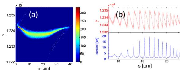
Figure 2: (a) Longitudinal phase space at the end of the linac. (b) Longitudinal phase space and the corresponding current distribution at the end of the ESASE section.
