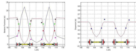
Figure 8: (Left) measured  $\beta_x$  (black) and (green),  $\beta_y$  (pink) and (red) at QF and QD respectively compared to theoretical ones in red and blue. (Right) measured dispersion (blue) compared to the theoretical one (red).
