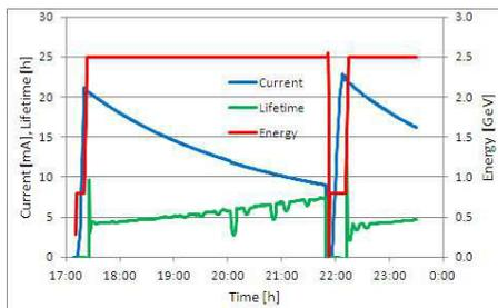
Figure 6: Machine filling and ramping cycle showing beam current and lifetime behaviour versus time.
