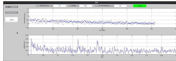
Figure 3: Measured ring tunes  $Q_x = 7.23$ ,  $Q_y = 6.17$ .
