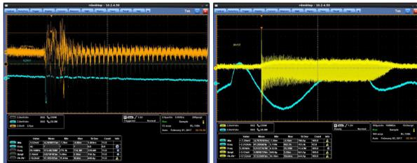
Figure 2: Ring FCT signals showing tens of beam turns with sextupoles OFF (left) and thousands of turns with sextupoles ON (right).
