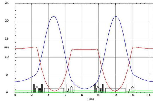
Figure 1: Optics 1 of SESAME storage ring showing betatrons  $\beta_x$  (red),  $\beta_y$  (blue) and dispersion  $\eta_x$  (green).
