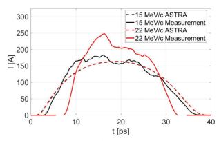
Figure 2: Beam current profiles of the optimized 4 nC beams. Note that the profiles from ASTRA are for the beams at Z = 5.28 m.
