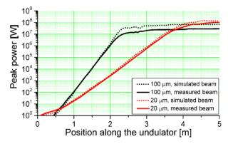
Figure 4: Simulated FEL peak powers along the undulator axis.
