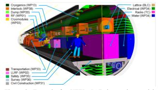
Figure 2: Example for XFEL CAD integration model, listing the contributions and their owning groups.
