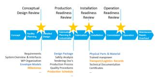
Figure 5: Project lifecycle with engineering reviews and examples for their content. Colors indicate the evolution of engineering design and schedule.
