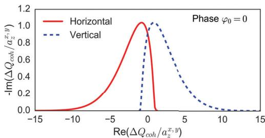
Figure 1: Stability diagrams for an rf quadrupole (second order) with  $\varphi_0 = 0$  for the two transverse planes. It was determined by solving the dispersion relation for detuning with longitudinal amplitude numerically [7].
