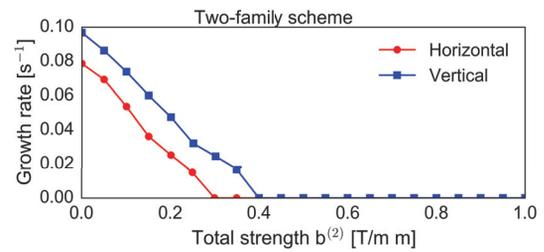
Figure 3: FCC-hh simulations for a two-family rf quadrupole scheme. Horizontal (red) and vertical (blue) growth rates are shown as a function of the *total* quadrupolar strength.
