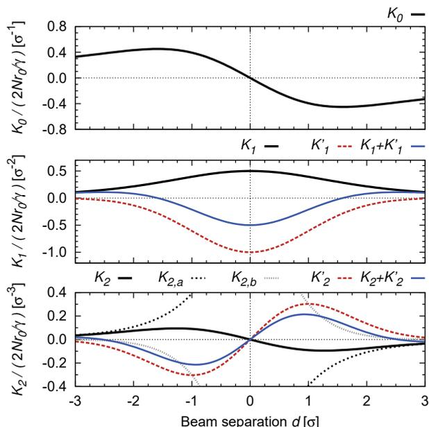
Figure 1: Dipolar (*top*), quadrupolar (*center*), and sextupolar (*bottom*) terms in the LR kick multipolar expansion.
