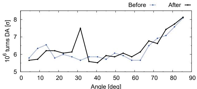
Figure 3: Dynamic aperture in the LHC before and after correction of HO and LR beam-beam at IP1 and IP5 (2 units of chromaticity,  $I_{\text{oct}} = 0 \text{ A}$ ).
