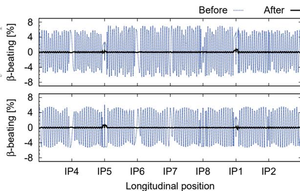
Figure 2: Beta-beating due to HO and LR beam-beam at IP1 and IP5 in the LHC before and after correction.
