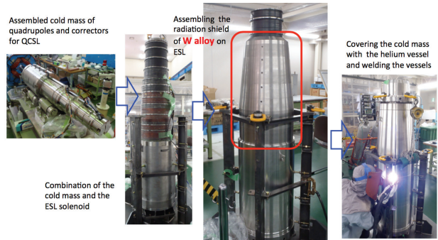
Figure 10: The construction of QCS (II).
