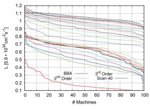
Figure 3: Tuning results for single beam case study. Each curve is the accumulated luminosity histogram obtained for 100 machines after every scan.
