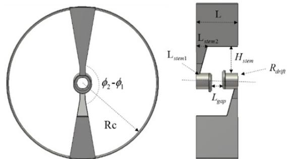
Figure 1: Primary geometry of single IH-DTL cell (left: front view, right: side view).
