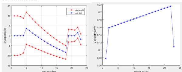
Figure 5: Phase and effective voltage variation along gap number.
