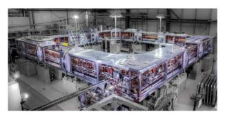
Figure 1: The cryogenic storage ring CSR with 35 m circumference.
