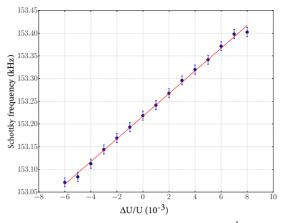
Figure 2: Schottky frequency measured at  $10^{th}$  harmonic of the revolution frequency as a function of the variation of the voltages of all CSR deflectors and quadrupoles expressed by  $\Delta U/U_0$ .
