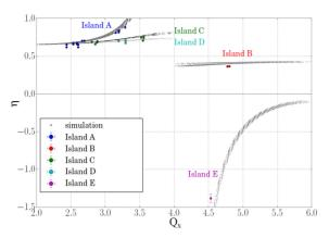
Figure 3: The measured (markers with error bars) and simulated (gray markers) phase slip factors for the cryogenic storage ring CSR as a function of the measured and simulated horizontal tune  $Q_x$ , respectively.
