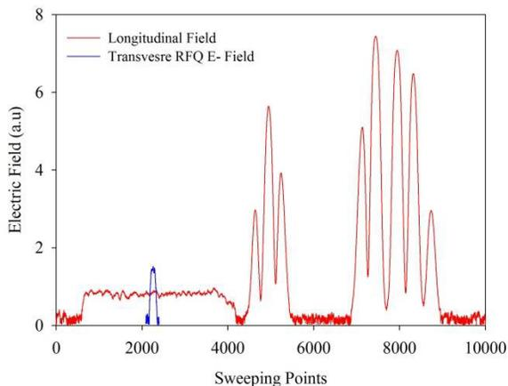
Figure 8: The on axis longitudinal electric field for the RFQ and IH-DTL (red) and the transverse RFQ electric field as measured in Figure 9.
