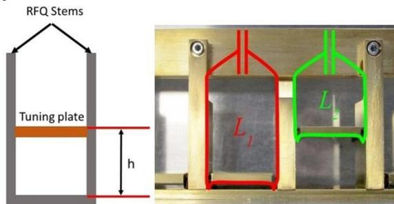
Figure 3: The tuning plate concept for RFQ tuning.
