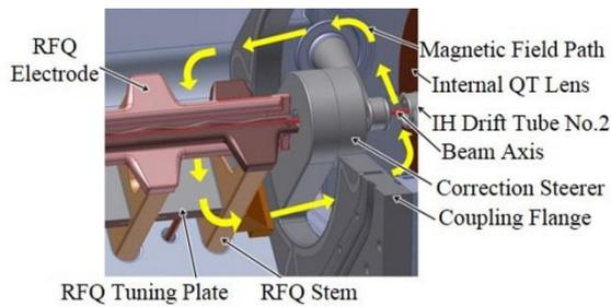
Figure 2: Detailed view for the inductive coupling between RFQ and IH-DTL including the correction steerer.
