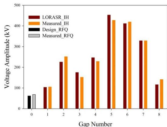
Figure 10: The measured effective gap voltage from bead-ball measurements versus the design gap voltage from the beam dynamics.
