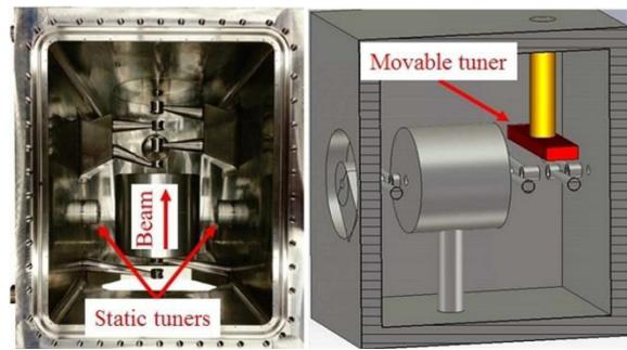
Figure 4: The position of the static and movable tuners for the IH-DTL cavity.
