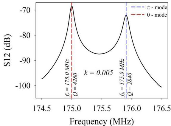
Figure 7: The 0 – and  $\pi$  – mode resonances for the coupled RFQ-IH-DTL structure.
