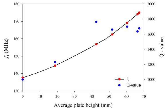
Figure 5: The resonance frequency and the quality factor versus the average height of the tuning plate for the RFQ.
