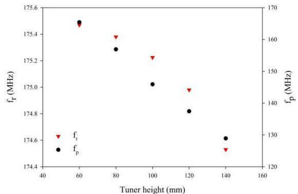
Figure 6: The resonance and plunger frequency in case of IH-DTL versus the movable tuner height and at an optimized static tuners shape.
