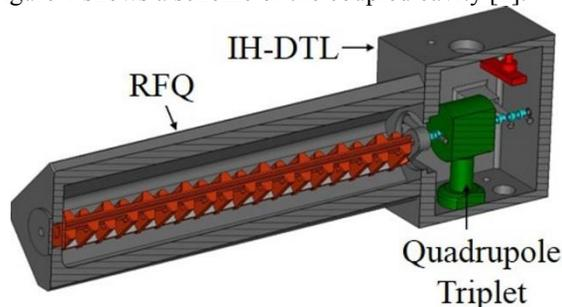
Figure 1: A 3D model for the coupled RFQ-IH-DTL cavity.
