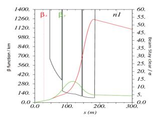
Figure 3: Example Plot Showing  $\beta$  Functions and Beam Stay Clear for Maximum FOM Triplet.
