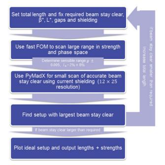
Figure 5: Outline of Triplet Optimisation Code used for an Alternative Triplet in FCC-hh.
