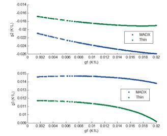
Figure 2: Predicted and Matched Quadrupole Strengths for Maximum FOM Configurations with Different Strength Outer Quadrupole.
