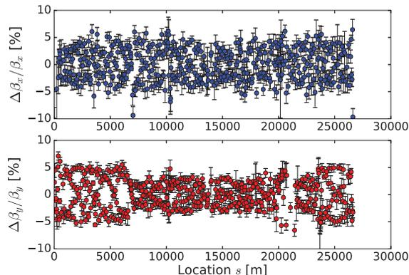
Figure 5: Measured  $\beta$ -beating for  $1.8\sigma_x$  and  $1.84\sigma_y$  amplitude particle due to beam-beam interaction at IP1 along the machine computed from BPMs data. This case corresponds to the AC dipole excitation shown on Fig. 3 and to the green plot on Fig. 4. The longitudinal coordinate starts at IP3.
