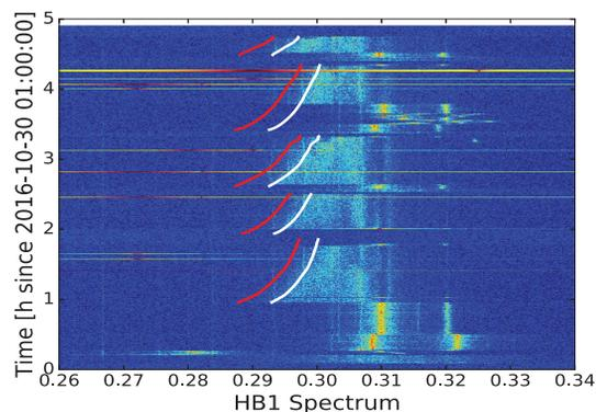
Figure 2: Horizontal Beam 1 spectrum from BBQ as a function of time during the MD. The red and white curves represent the tune shift due to beam-beam collision, i.e.  $Q_x - \xi_x$ , based on the measured emittance and if a 20% larger emittance is assumed respectively.
