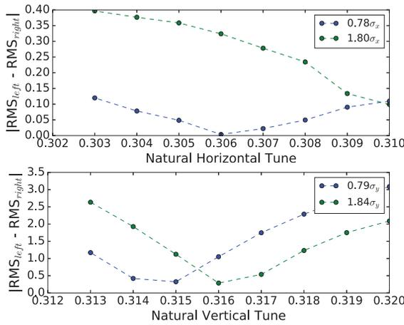
Figure 4: Horizontal (top plot) and vertical (bottom plot) scan of the natural tune where the RMS of the  $\beta$ -beating was computed for two different AC dipole excitations.
