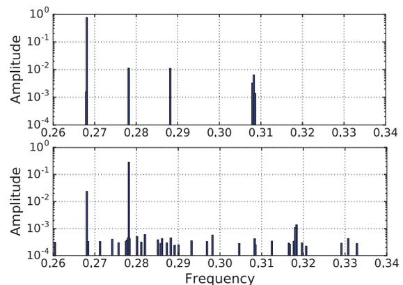
Figure 3: Horizontal (top) and vertical (bottom) Beam 1 spectra for AC-dipole excitation with  $1.8 \sigma_x$  and  $1.84 \sigma_y$  respectively. Excitation frequencies were  $f_{\text{excit}} = (0.268, 0.278)$  and the value of the natural tunes seen on the spectra are (0.307, 0.317) on the x-y plane.
