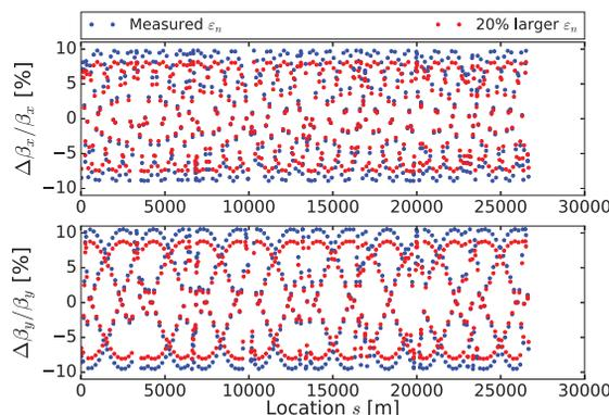
Figure 6: Simulation of  $\beta$ -beating in the LHC due to head-on beam-beam interaction at IP1 at injection energy for zero amplitude particles. Blue points were computed based on the measured normalized transverse emittance and the red ones assuming a 20% larger emittance. The longitudinal coordinate starts at IP3.
