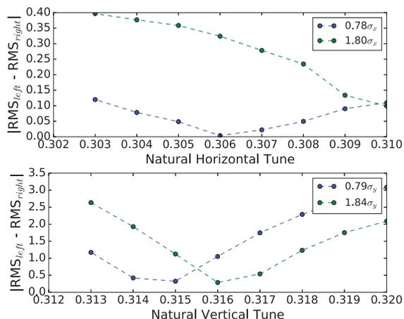
Figure 4: Horizontal (top plot) and vertical (bottom plot) scan of the natural tune where the RMS of the  $\beta$ -beating was computed for two different AC dipole excitations.
