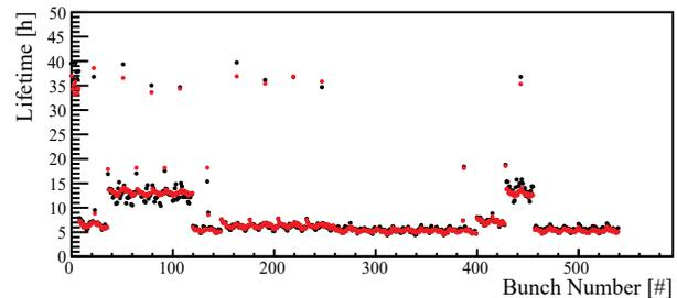
Figure 6: Fill 5549: bunch lifetimes along the train, from measured data (black) and the corrected ODE model (red).
