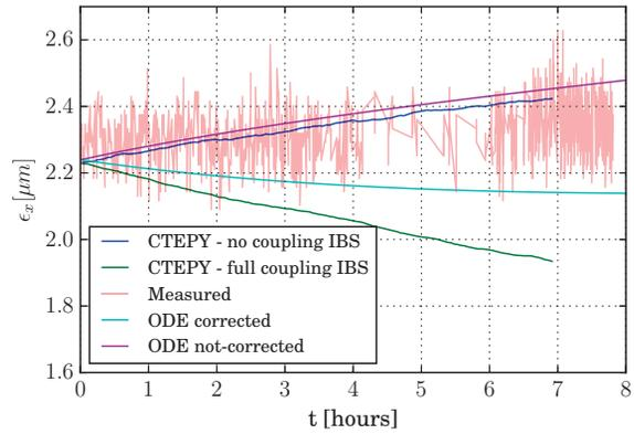
Figure 4: Fill 5549; Horizontal (normalized) emittance evolution bunch 5.
