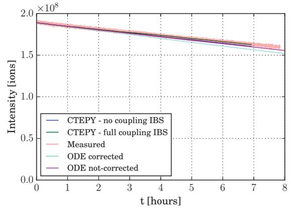
Figure 1: Fill 5549; Intensity evolution bunch 5.
