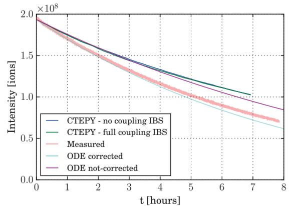
Figure 2: Fill 5549; Intensity evolution bunch 73.
