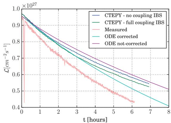
Figure 5: Fill 5549; Luminosity at IP5 for bunch 73.
