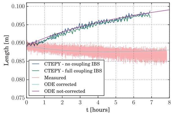
Figure 3: Fill 5549; Bunch length evolution bunch 5.
