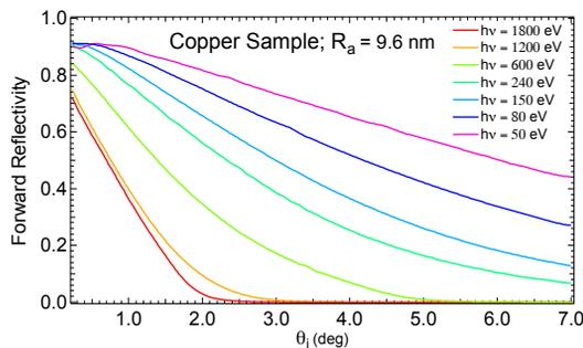
Figure 5: Measured normalized reflectivity vs. incidence angle for different energies for a copper surface, for different photon energies.
