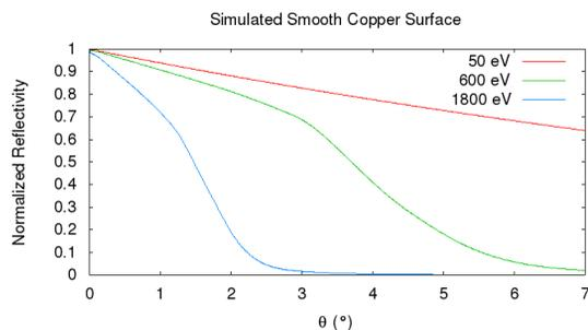
Figure 6: Simulated normalized total reflectivity vs. incidence angle for different energies for a copper surface, for different photon energies.
