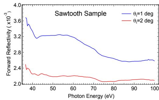
Figure 7: Measured normalized forward reflectivity as a function of the energy of impinging photons (36 eV - 100 eV), for two different incidence angles on a sawtooth chamber.
