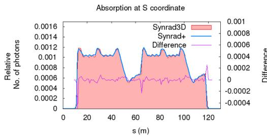
Figure 1: Simulated photon absorption as a function of longitudinal coordinate  $s$  for one LHC arc cell, treating the chamber wall as a perfect absorber; the blue line is the result using Synrad+, while the red area is the result from Synrad3D.
