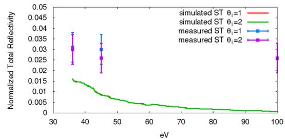
Figure 8: Simulated normalized total reflectivity as a function of the energy of impinging photons (36 eV - 100 eV), for two different incidence angles on a sawtooth chamber.
