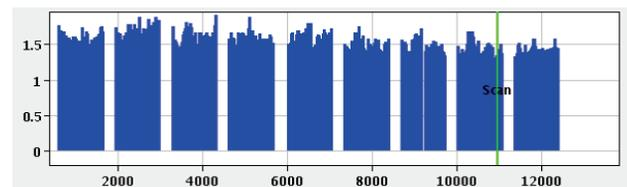
Figure 4: Vertical normalised emittance for several injections of bunch trains with 800 ns batch spacing.
