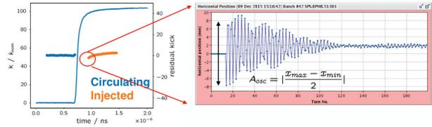
Figure 1: Using bunch-by-bunch and turn-by-turn beam position data to optimize the kicker system timing.
