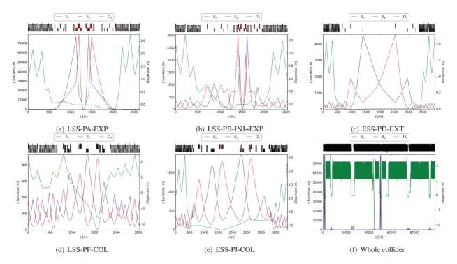
Figure 3: Optical functions of the insertion regions at collision: high-luminosity IR, low-luminosity IR with injection, extraction section, betatron and momentum collimation section.
