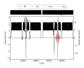
Figure 4: Closed orbit and dispersion in the ring after correction of the spurious dispersion in presence of the crossing scheme.
