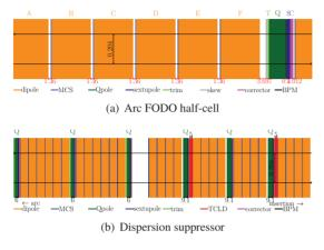
Figure 2: Layout of the arc FODO half-cell and DIS.
