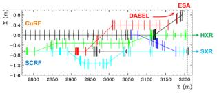
Figure 4: Top view of the spreader area, where the DASEL beamline and components are colored in red. Note that different lines may be at different elevation.
