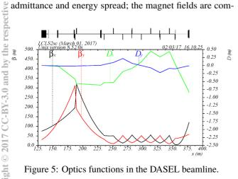
Figure 5: Optics functions in the DASEL beamline.
