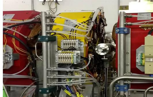
Figure 1: Sextupole magnet (yellow) with corrector installed on DDBA cell.
