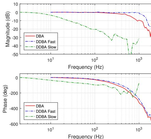
Figure 5: Measured vertical frequency responses of a DBA corrector magnet (—), a fast DDBA corrector (---) and a slow DDBA corrector (---).
