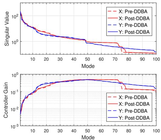
Figure 4: The top plot shows the singular values pre-DDBA for the X-axis (---) and Y-axis (---) compared to the singular values post-DDBA for the X-axis (—) and Y-axis (—).
