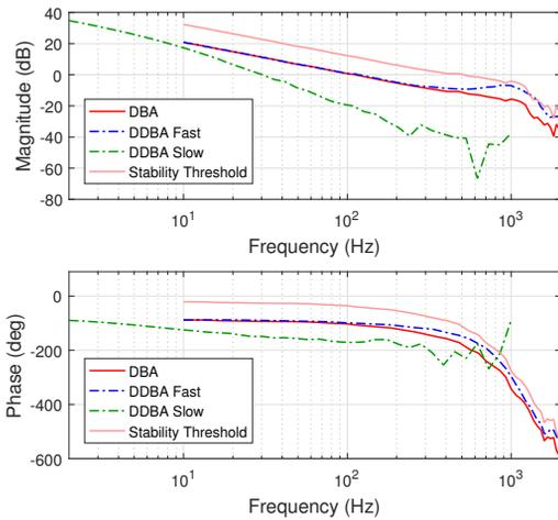
Figure 6: Measured vertical frequency responses of the forward control loop for a DBA corrector magnet (—), a fast DDBA corrector (---) and a slow DDBA corrector (- -). The gain and phase margins are also shown (-).
