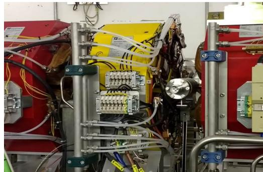
Figure 1: Sextupole magnet (yellow) with corrector installed on DDBA cell.
