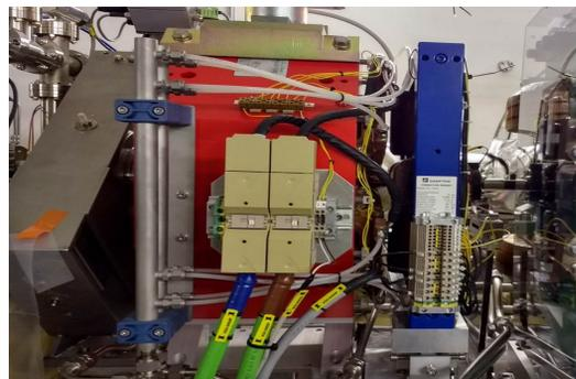
Figure 2: Discrete corrector (blue) installed on DDBA cell
