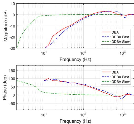
Figure 7: Measured vertical sensitivities of a DBA corrector magnet (—), a fast DDBA corrector (---) and a slow DDBA corrector (- -).
