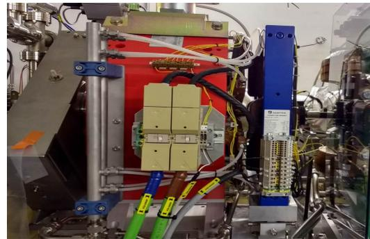
Figure 2: Discrete corrector (blue) installed on DDBA cell
