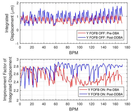
Figure 8: The top plot shows the integrated vertical beam motion ( $\mu\text{m}$ ) up to 100 Hz pre-DDBA (—) and post-DDBA (---). The bottom plot shows the factor by which the integrated beam motion was suppressed with FOFB pre-DDBA (—) and post-DDBA (---).
