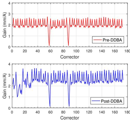
Figure 3: The top plot shows the maximum gain (mm/A) of the response matrix for each corrector pre-DDBA (—) and the bottom plot shows the same post-DDBA (—).
