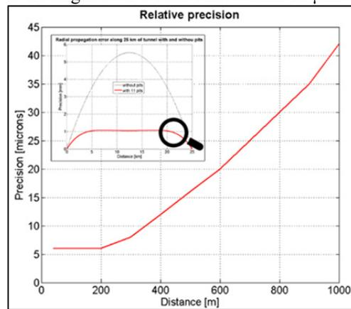
Figure 7: relative precision to the stretched line according to the distance considered.
