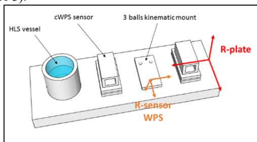
Figure 3 : Configuration of TT1 metrological plate.
