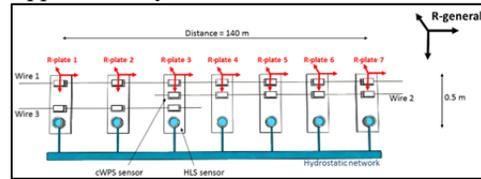
Figure 4 : Configuration of the 140 m facility.
