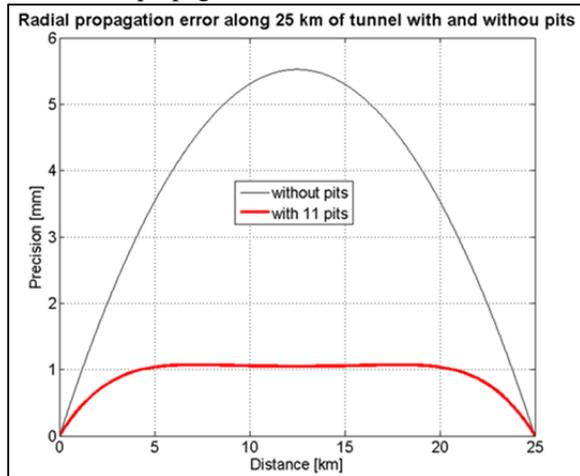
Figure 6: radial propagation error along a 25 km of tunnel with/without pits.
