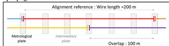
Figure 1: Configuration of overlapping stretched wires.
