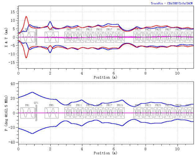
Figure 4: Envelope before cavity failure.
