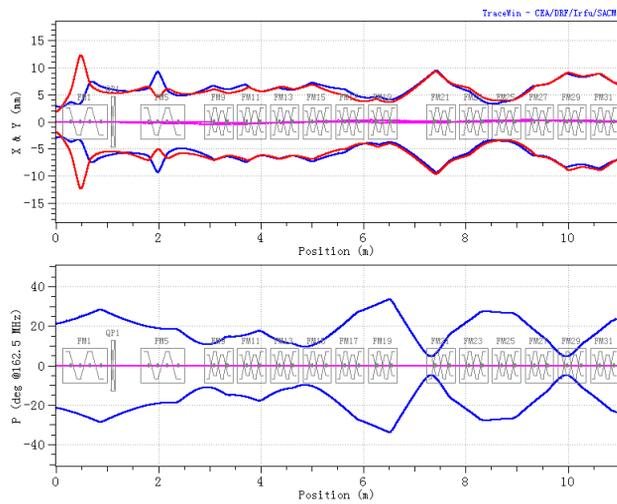
Figure 6: Envelope after the fourth cavity failure.
