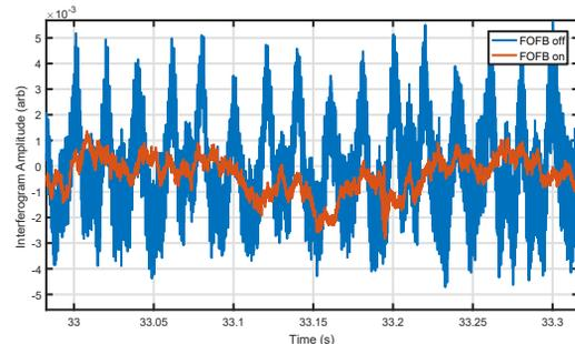
Figure 7: FarIR beamline’s interferometer data showing a significant reduction in the 50 Hz noise.
