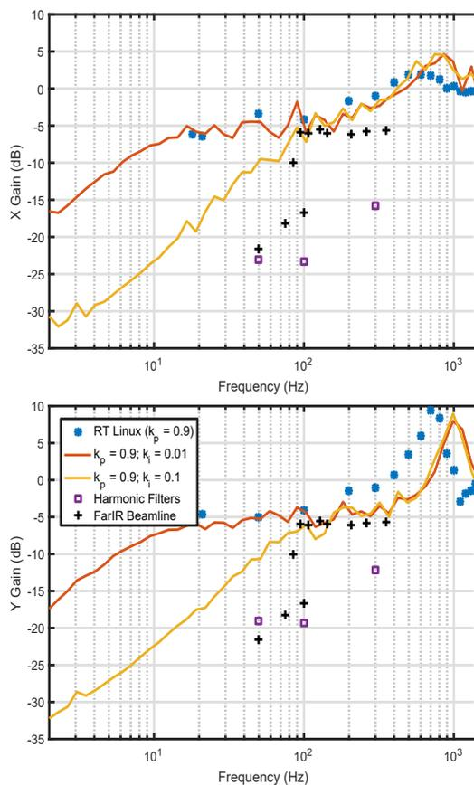
Figure 4: A comparison of the closed loop gain\* of the PC and FPGA based feedback system. We also show the effect of different integral gain coefficients and effectiveness of the harmonic suppressors.
