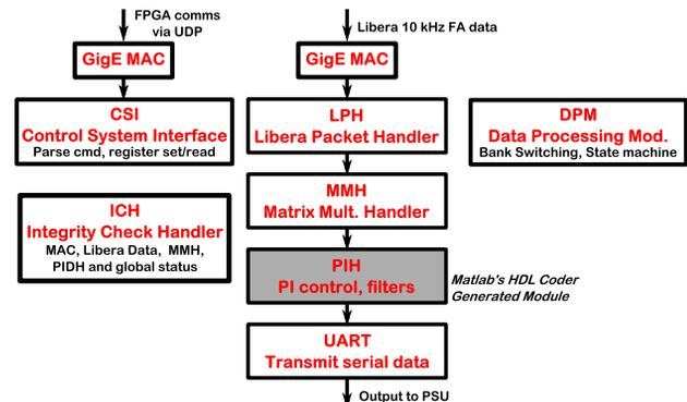
Figure 2: Simplified system architecture developed by Arrayware and AS.
