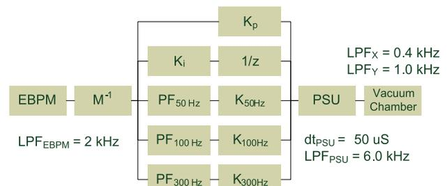
Figure 3: Controller for the FOFB where the harmonic suppressors are implemented using 2<sup>nd</sup> order IIR peak filters (biquad filters in direct form 2).
