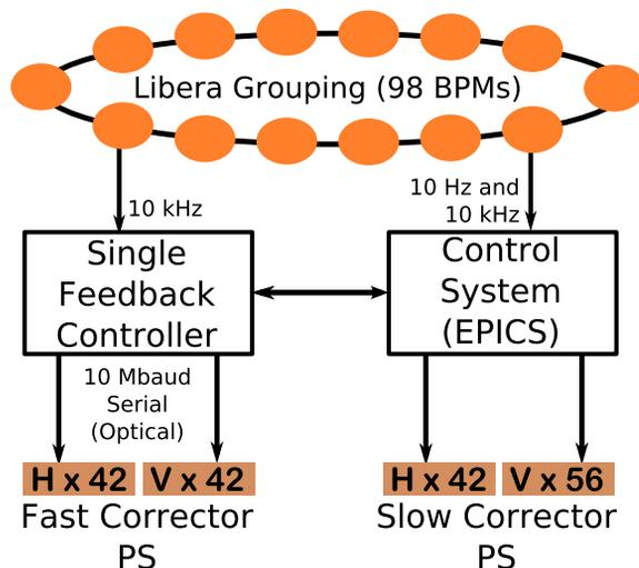
Figure 1: FOFB system with a single feedback controller controlling the fast corrector power supplies.
