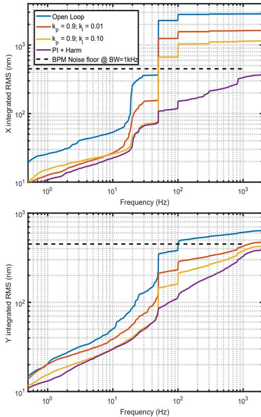
Figure 5: Integrated RMS showing that the FOFB is now damping beam motion down to the noise floor of the BPMs which is at 450 nm for a bandwidth of 1 kHz.
