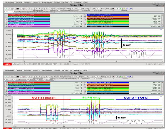
Figure 6: The effect of an APPLE2 undulator scanning in elliptical polarisation mode. Horizontal (top) and Vertical (bottom) beam position (10 Hz BW) is monitored showing significantly improved orbit stability in the presence of moving insertion devices.
