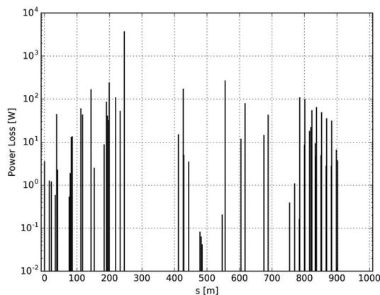
Figure 4: Inelastic proton power loss map per element.
