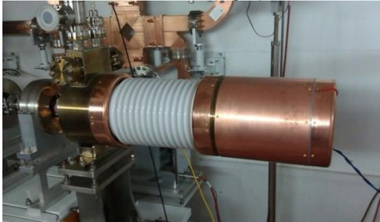
Figure 4: Triode electron gun of the NSC KIPT 100 MeV/100 kW linear accelerator.
