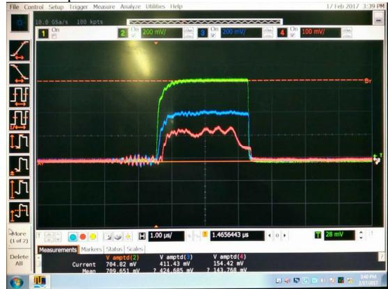
Figure 6: Profile of the electron beam along NSC KIPT 100 MeV/100 kW linear accelerator. Green – after electron gun, Blue – after the electromagnetic chicane, Red – after the first 45 degree transportation channel bending magnet.
