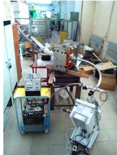
Figure 3: Testing of the transportation channel vacuum claps at vacuum bench.
