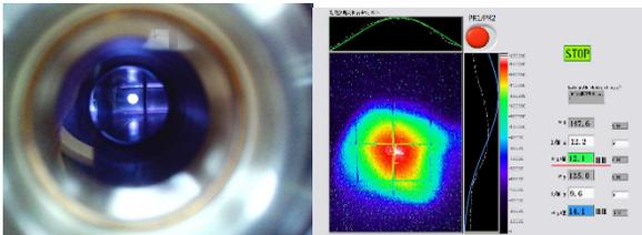
Figure 5: Electron beam at electron gun exit during injection section commissioning (0.5 A).
