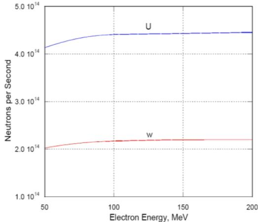
Figure 2: Neutron source flux vs electron energy for 100 kW electron beam power of natural uranium and tungsten target materials.
