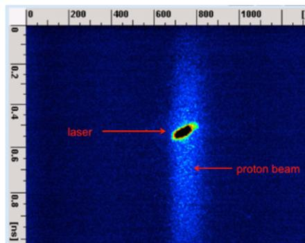
Figure 6: Streak camera measurement in a 1 ns time window for the laser and proton synchronisation. The short laser pulse is centred longitudinally on the long proton bunch.
