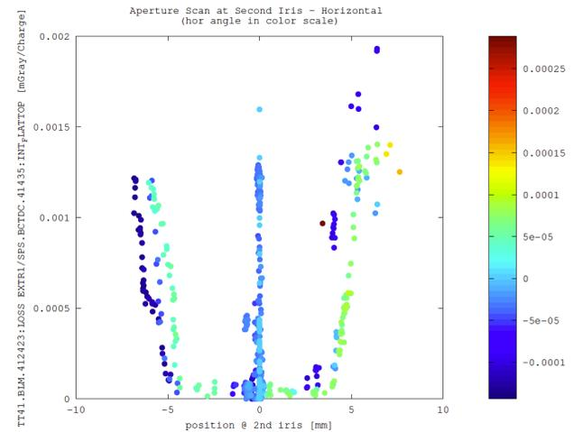
Figure 4: Example for a position scan of the plasma cell irises. The plot shows the normalised beam loss with respect to the beam position. The beam angle (in the colour scale) allows to distinguish losses at the first or second iris.
