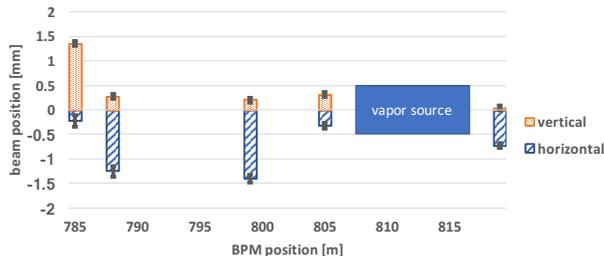
Figure 5: Measured reference beam positions for the proton beam downstream of the laser merging point. The trajectory has been optimised to be centred in the plasma cell irises.
