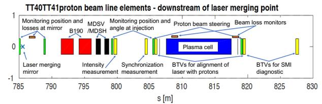
Figure 3: Set up of the last magnetic elements (B190 dipoles and MDSV, MDSH corrector magnets) and beam instrumentation downstream of the laser merging mirror.
