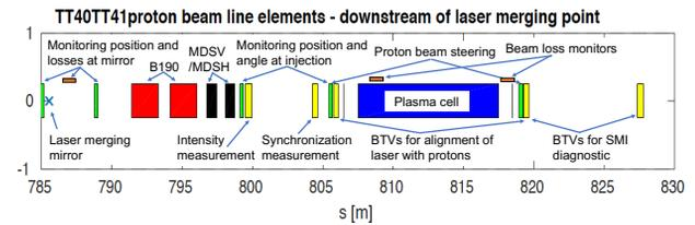
Figure 3: Set up of the last magnetic elements (B190 dipoles and MDSV, MDSH corrector magnets) and beam instrumentation downstream of the laser merging mirror.
