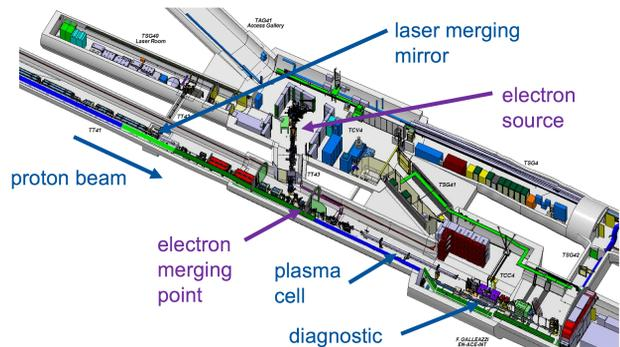
Figure 1: View of the AWAKE facility. The proton and laser beam are installed together with the plasma cell and SMI diagnostic for phase1, which has started in 2016. One year later, the electron beam line and additional diagnostics will be added for phase2.
