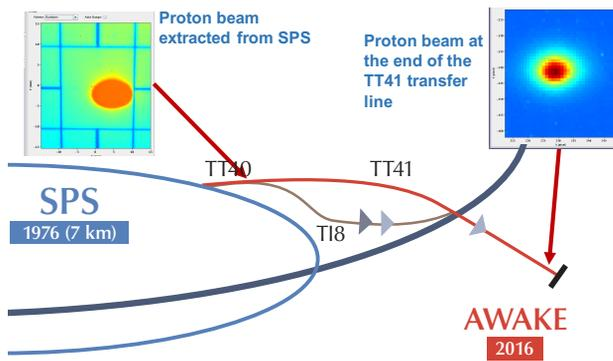
Figure 2: Proton beam profiles taken during the first beam time for AWAKE in June 2016. The beam is imaged on two BTV screens, one just following the SPS extraction channel and one at the end of the TT41 beam line.
