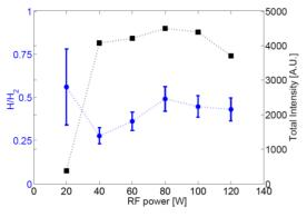
Figure 3: Dependence of the  $n_H/n_{H_2}$  ratio on RF power.
