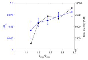
Figure 5: Dependence of the  $n_H/n_{H_2}$  ratio on the B<sub>max</sub>/B<sub>min</sub> ratio.
