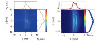
Figure 5: Left: Measured intensity on the fluorescent screen at the end of the whole beam transport line as measured in [3, 4]
