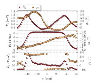
Figure 1: Results of the circular magnetic field measurements of QG1. Shown are the first three multipole strengthes  $\hat{F}_{n=1,2,3}$  and the according phases  $\varphi_{n=1,2,3}$  along the nominal beam axis. The yokes reach from  $\pm 40$  mm.
