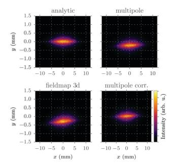
Figure 2: Simulated beam profiles for a bunch with gaussian distributed momentum and divergence for the three different quadrupole models and the corrected multipole model, each focusing in the *y*-plane.
