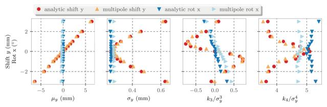
Figure 4: Comparison of the statistical moments of the particle distribution on the simulated beam screen for different misalignments between the analytical and multipole magnet models.
