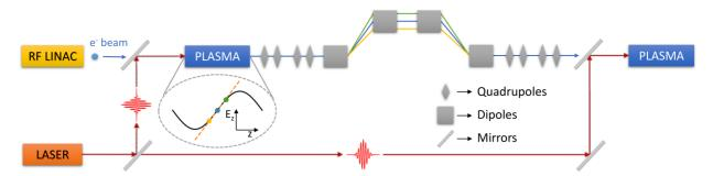
Figure 1: Schematic view of the synchronizing stage.
