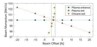
Figure 4: Jitter correction thanks to plasma stage and chicane. The vertical lines delimit a 1 fs jitter.
