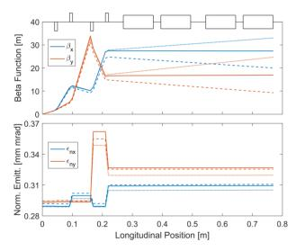
Figure 3: Beta function and emittance evolution for beams with different offsets. The solid line corresponds to  $\Delta \xi_i = 0$ , while the dashed and dotted lines represent offsets of 20 and -20 fs, respectively.
