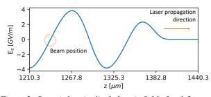
Figure 2: On-axis longitudinal electric field after 1.2 mm of propagation in the plasma with the electron beam placed at the zero crossing (case with  $\Delta \xi = 0$ ).
