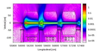
Figure 4: Elevation map at beam plane of the total fluence per mis-steered electron  $[cm^2/e^-]$  in the first three segments down-beam of the 1 mradian vertical mis-steering
