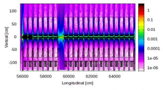
Figure 5: Elevation map at beam plane of the total fluence per lost electron along SXR beam-line [cm<sup>2</sup> /e<sup>-</sup>]
