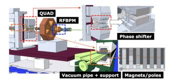
Figure 1: Flair [4] visualization of the models of LCLS-II SXR undulator, phase shifter, RFBPM, as implemented in FLUKA
