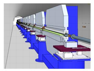
Figure 2: Rendering of the LCLS-II SXR undulator beamline as implemented for these studies
