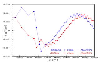
Figure 3: Simulated and theoretical transverse positions along SXR for  $30 \,\mu m$  initial offset in either plane
