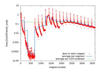
Figure 6: Absorbed dose in the individual magnets (red), in all magnets of each segment (blue), or in the entire set of SXR undulator magnets (green) per each 100 bunch beam scan ([Gy/scan])
