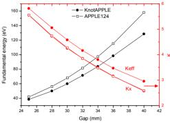
Figure 5: The gap-dependent of the fundamental energy and *K*. The Knot-APPLE (solid circle) and APPLE124 (open square).
