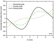
Figure 7: Horizontal second-order kick (eq.3) for the Knot-APPLE in the mid plane for horizontal (dotted), circular (dashed) and vertical (solid) polarization.
