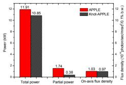
Figure 3: Comparison of APPLE124 and Knot-APPLE parameters. The bar chart shows the total power, the partial power and the on-axis flux.
