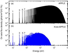
Figure 2: Comparison of the on-axis angular flux density spectra for the APPLE124 (a) and the Knot-APPLE (b), both with a period length of 124 mm. Indices show the harmonic number.
