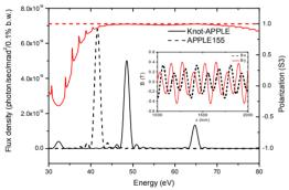
Figure 6: Angular flux density and degree of circular polarization for the Knot-APPLE (solid line) and APPLE155 (dashed line). The insert shows the magnetic field distribution in the Knot-APPLE.
