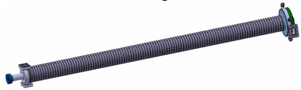
Figure 2: Full two-meter long gun, the cathode and the power input are on the left side.
