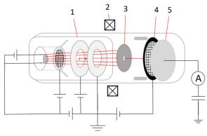
Figure 4: Schematic of test bench. 1 electron gun; 2 FCT; 3 beam scraper; 4 decelerating grid; 5 collector.
