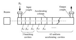
Figure 3: Schematic diagram of the accelerating tube.
