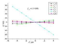
Figure 2: RF frequency changing rates with different cavity dimensions.
