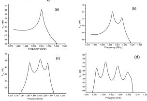
Figure 8: Testing result of cavities. (a) refers  $S_{21}$  curves of one and two half cavities; (b) refers two and two half cavities; (c) is three and two half cavities; (d) is four and two half cavities.
