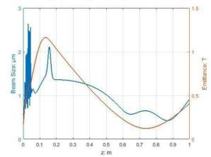
Figure 6: Evolution of emittance and beam size with distance to the cathode.
