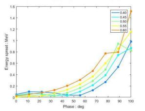
Figure 2: Energy spread with phase for guns with different length of first cell.
