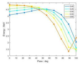
Figure 1: Energy changed with phase for guns with different length of first cell.
