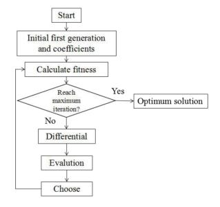
Figure 3: Flow chart of DE algorithm.
