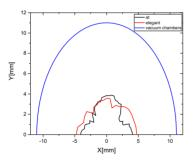
Figure 4: Dynamic aperture and physical aperture at the centre of the long straight section.
