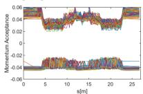
Figure 2: Momentum acceptance computed for 100 error sets.
