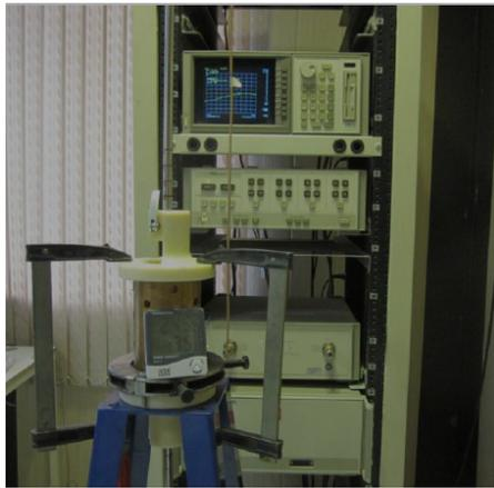
Figure 9: cell by cell Measurement and tuning of prototype.
