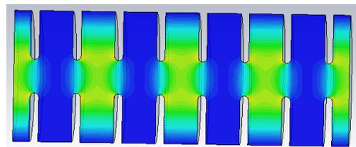
Figure 2: Electric field profile of  $\pi/2$  (CST Studio Suit).
