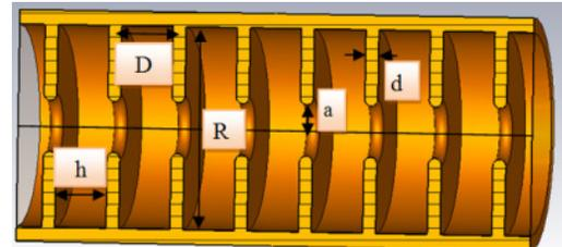
Figure 1: Geometrical parameters for design of constant impedance TW accelerator cavities.
