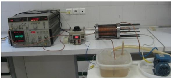
Figure 5: Experimental setup for measurement of frequency and quality factor and evaluation of them based on variation of temperature.
