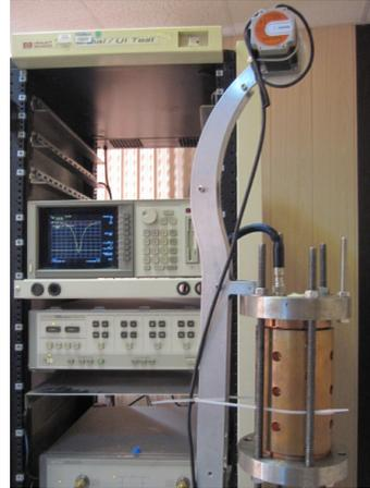
Figure 8: Attached bead pull system on prototype 9 cells cavity.
