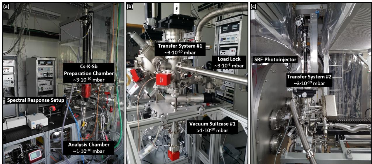
Figure 3: The bERLinPro photocathode infrastructure: (a) Preparation and Analysis System with spectral response setup. (b) Transfer system #1 with load lock and Vacuum Suitcase #1. (c) Transfer system #2 at the SRF-photoinjector.
