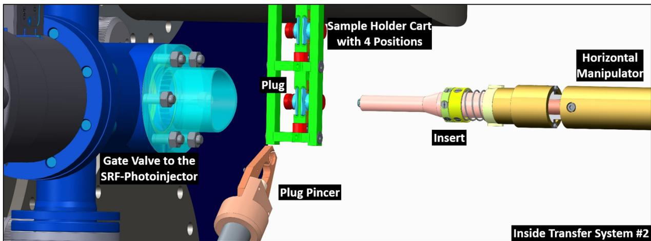
Figure 4: A reduced 3D model of the inside view of transfer system #2 attached to the SRF-photoinjector module.
