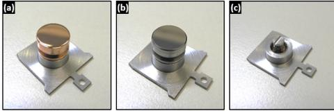
Figure 2: The flag style sample holder system with: (a) polycrystalline Cu plug for initial commissioning of the SRF-Photoinjector. (b) a polycrystalline Mo plug used as substrate for Cs-K-Sb photocathodes. (c) an empty sample holder to show the CuBe spring holding the plug.
